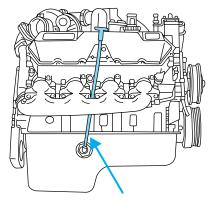
5. Read oil level on both sides of dipstick and use highest level (reading) for the actual engine oil level.
